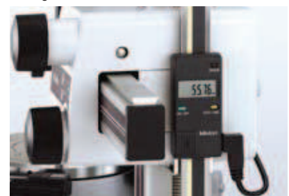
Continuous inside and outside diameter function (outside dia. surface)
